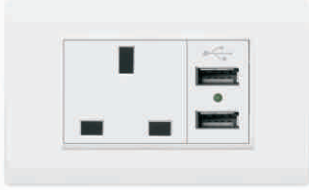
118BS-12 10-20A 110-250V~ 50/60Hz 5V 2100mA 13A square pin socket+ USB
